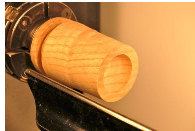
Bottom partially hollowed and ready for fitting tenon to mortise in lid
