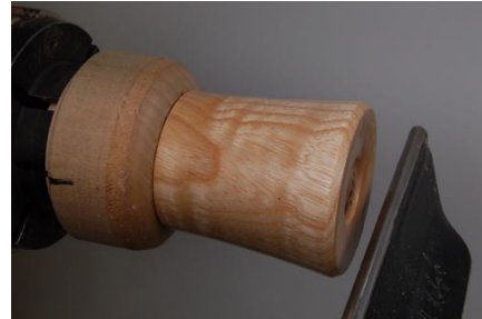
Bottom fitted in jam chuck using a mortise in the jam chuck so that bottom can be turned and detailed
