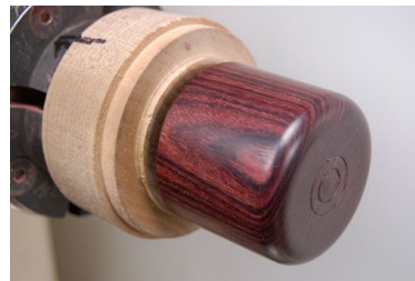
Bottom fitted into jam chuck using a tenon to fit the inside of the box
