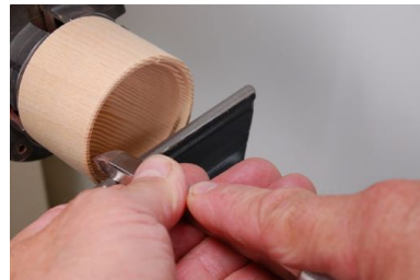
Using Box Tool to cut in mortise
