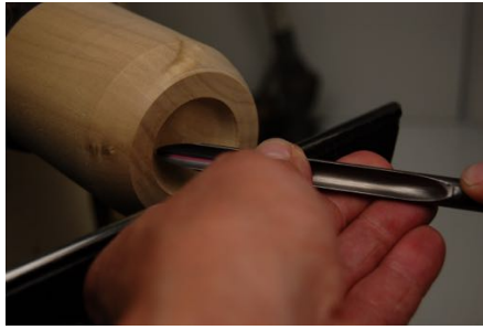
Hollowing with 3/8" Spindle Gouge
