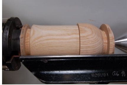
Top fitted to bottom with tail stock pulled up for extra support until ready for final cut
