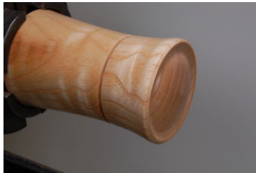
Lid attached and ready for finishing cut and sanding
