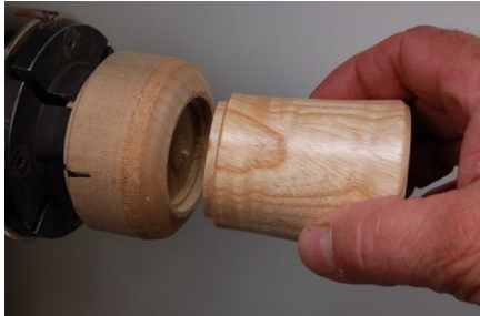
Bottom fitted in jam chuck using a mortise in the jam chuck so that bottom can be turned and detailed
