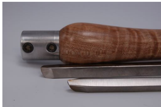
Top & Side view of Box Scraper with Handle & Collet
