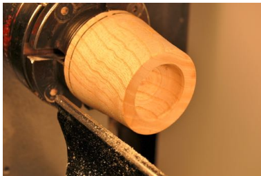
Top of the box partially hollowed ready for cutting in mortise
