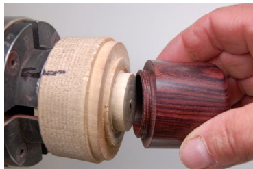
Bottom fitted into jam chuck using a tenon to fit the inside of the box
