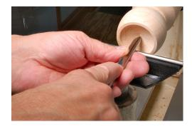
10. With the flute of the gouge in the fully open position, push the tip into the blank approximately ¼". Now rotate the flute toward you, to the 11 o'clock position, push the cutting tip toward the outside while pushing the handle down and dragging the cutting edge out. The idea is to remove as much wood as quick as possible. With each cut the hole being created is getting wider as well as deeper.
