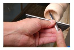
Note: Remember the goal here is to open up the bowl area so that a round nose scraper can be used to finish hollowing the inside of the bowl.
