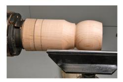
Tip: Do not turn the bottom of the bowl all the way down to the stem. Leave extra wood at the base of the bowl to help provide stability when hollowing the end grain, as end grain hollowing, is very aggressive and the bowl of the goblet will need the extra support.
