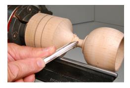
16. Shape the base keeping it in proportion to the top of the goblet. The base should be slightly larger than the diameter of the top. To insure that the finished goblet does not look like it will fall over and that the goblet looks well proportioned.
