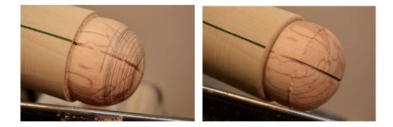
\*Note in the photo above left I have used a pencil to mark the area where I still need to remove a bit of material. The photo on the right shows the sphere after it has be reversed to turn the other half down to the pencil line.
