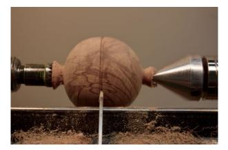
10. Once the sphere has been roughed out use a thin parting tool to make a shallow dado or channel at the center line on the sphere and then using a pencil remark the center line before paring parting it off the lathe. Be sure to leave little nubs on the ends just in case the extra wood is needed for the final shaping of the sphere.
