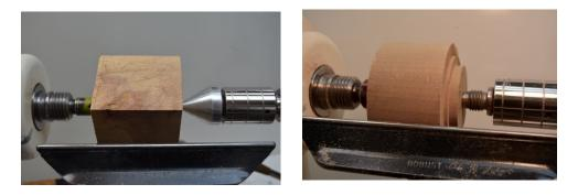
2. Place the blank that is to be the sphere in the chuck and true up the blank.
