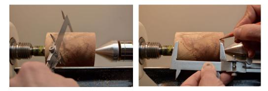
**3.** Next measure the diameter of the cylinder with a pair of Venier Calipers (if turning a sphere to a specific diameter turn the blank to a diameter slightly larger than the finished diameter to allow for final shaping and sanding) and transfer this measurement to the side of the blank leaving some room for waste on both ends, in order to insure that there is room for the tools to get around to turn the sphere shape without hitting the drive center or the revolving center.
