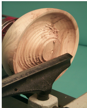
Hollowing a large bowl using the stair stepping method leaving material in the center of bowl to minimize flexing of outside of bowl
