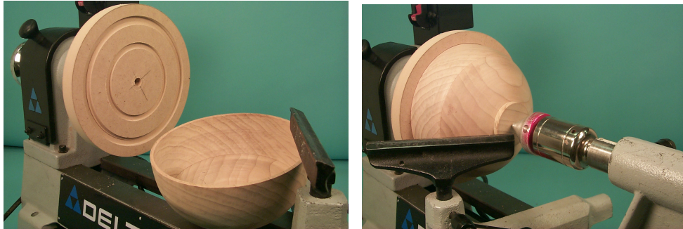
MDF mounted in a 4 Jaw Chuck or on a faceplate with grooves for jam chucking bowl rims for reverse turning
