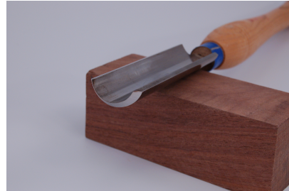
1 1/4" Continental Gouge ground straight across with 40 degree bevel
