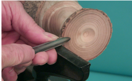
The facing cut with flute fully closed at 3 O'clock
