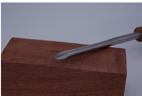
3/8" Spindle Gouge with 35 degree bevel with the wings ground back
