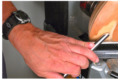
Pull cut in shear scraping position handle at 45 degrees
