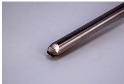
Traditional ground bowl gouge with convex relief and micro bevel at 40 degrees
