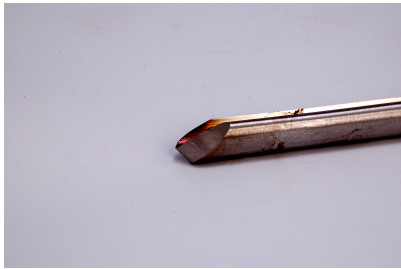
Side ground bowl gouge 50 Degree bevel
