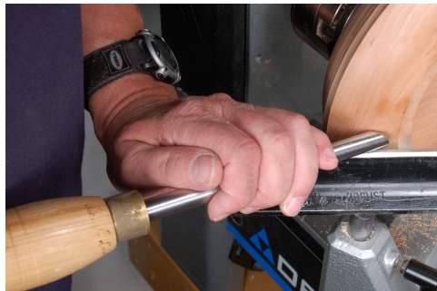
Pull cut in horizontal scraping position
