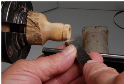
Begin chasing the male threads with the tool starting at a 45 degree angle
