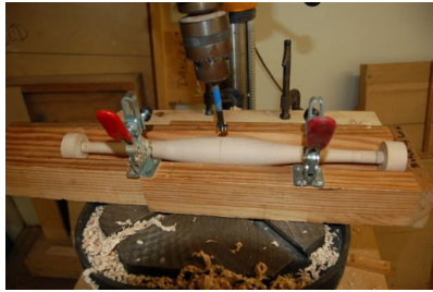
Tommy Boyd's jig for drilling mortises on a tilting head drill press
