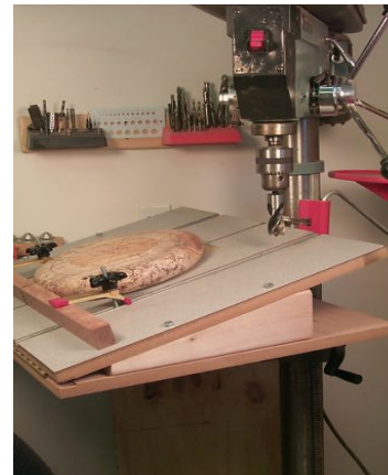
Adjustable drill press table for drilling holes in the seat
