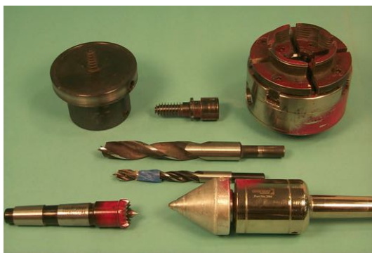
The chuck, drill bits, Steb center, screw & bearing center
