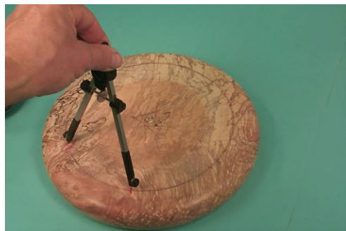
Photos of how I lay out and space the holes for the legs, using the radius of the circle to divide the circle with six arcs and then skipping every other arc mark them for drilling the leg holes
