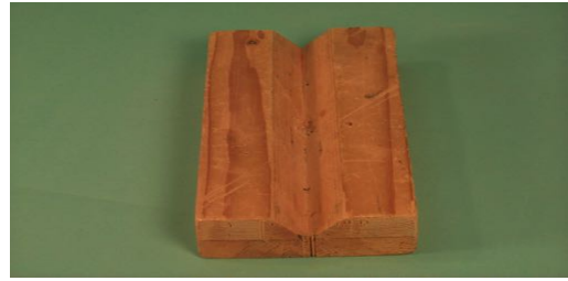
Photo of V Jig for cutting cylinders on the Band Saw & for cutting the slot in the leg for the wedge
