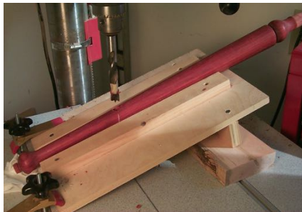
The old jig in use on the drill press
