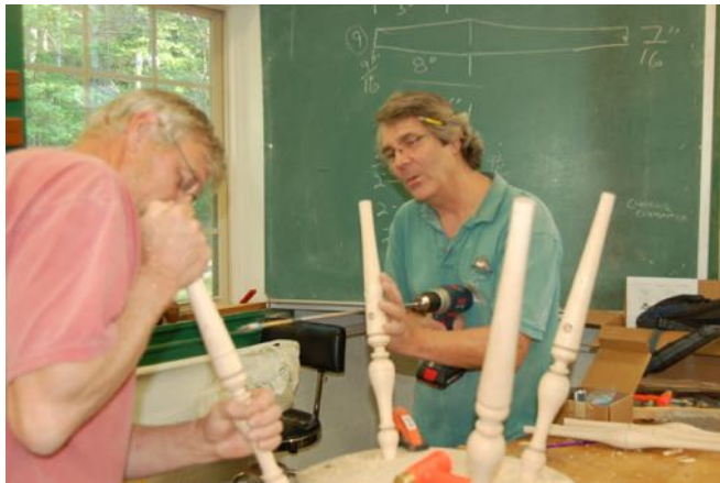
Using hand drill with spade bit to drill leg mortises
