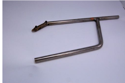
Swan neck Tool with adjustable angle settings
