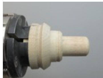
Jig for holding pepper mill bottoms after drilling
