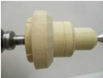
Jig for holding pepper mill bottoms after drilling
